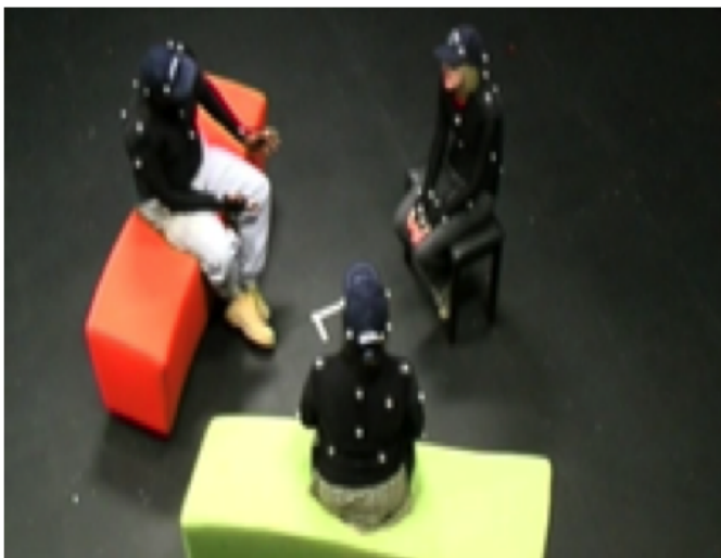
Figure 1: 2-dimensional image of participants engaged in triadic interaction, wearing the reflective markers
